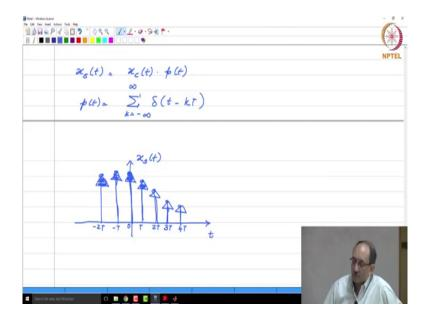
So, here we have the underlying continuous time signal. And now we are going to sample it using impulse train, which means, I now have this picture with me each of them is not just a number, but each of them is now an impulse. And the strength of the impulse is proportional to the value of the sample.
