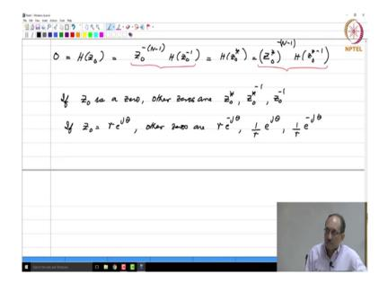
Therefore,  $H(z_0)$  will be  $z_0^{-(N-1)}H(z_0^{-1})$ . And because  $z_0$  being a zero means  $z_0^*$  also is a zero. So, if  $z_0$  were a zero,  $H(z_0) = 0$ . And  $H(z_0) = H(z_0^*)$  also because of symmetry, because the sequence is real. If  $z_0$  were a zero,  $z_0^*$  also is a zero. If  $z_0^*$  is a zero, then this must also be  $(z_0^*)^{-(N-1)}H((z_0^*)^{-1})$ .
