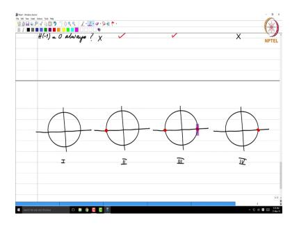
So, in the z-plane, so this is I, II, III and IV. So, type I, there is no constraint zero either at z = 1 or z = -1. Whereas, for type II, there is always a zero at -1. For type III, you have zeros both at z = 1 and z = -1. And type IV, you have a zero at z = 1. So, no matter what the coefficients are, you are guaranteed that these zeros will be present given the nature of symmetry of these sequences.
