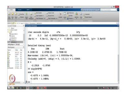
So, it gives me this values of K, right. And I can easily check what are the eigenvalues of A + BK and you can see that the closed loop system is actually stable, right, ok. So, this is some very very basic examples that you can try out discrete time version of this you can try out Schur complements and so on, but I will just leave that to you. It is just a matter of typing down; typing down the code, ok. A few more examples I would like you to quick, to quickly do here.
