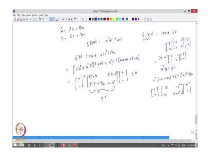
So, I have  $\dot{x} = Ax + Bu$ , y = Cx + Du, ok. My storage function S(x(t)) is say  $x^T Px$ , ok. Let me leave out the half for the moment, ok. Now, what I should find out is how does  $\dot{S}(x(t))$ -S(u,y)  $\leq 0$ , ok. So, first let us look at this term.  $\dot{S}$  is, so I get  $\dot{x}^T Px + xP\dot{x}(t)$ . This is, so this is  $(x^T A^T + u^T B^T)Px(t) + x^T(t)P(Ax(t)+Bu(t))$  So, this I can a club it in the following way. So, I have x u transpose x u.
