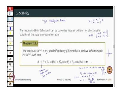
So, what is the LMI here? How do I check given a A matrix and given a certain D R region if that particular system represented by an A matrix is D R stable or not. So, one result that says, ok, this from a reference that is mentioned towards the end of the slides is that a matrix A is D R stable and this D R stable these regions are defined by this choice of matrices  $R_{11}$ ,  $R_{12}$ , and  $R_{22}$ .
