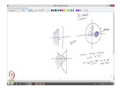
So, suppose, let us let us work in the discrete time case for the moment, that so I have x(k+1) = Ax(k) + Bu(k). The standard stabilization problem would be find control law u(k) = kx(k) such that the eigenvalues of A + BK are the eigenvalues are in the unit disk, right. And then we know now, how to first formulate this as an LMI that is what we learned in lecture number 1.
