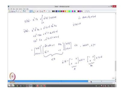
So, I have  $V(x(t)) = x^T Px + \int_{t-\tau}^{t} x^T(\tau) Sx(\tau) d\tau$  ok. Then I do the differentiation  $V(\dot{x(t)})$ . Again, along the system trajectories what are the system trajectories system trajectories are  $\dot{x(t)} = Ax + A_d x(t-\tau)$ , ok.
