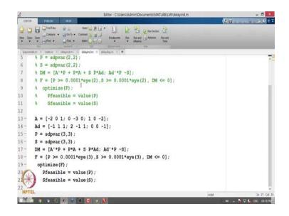
So, what I will be interested in is to solve is to check for stability of this particular delay system  $x(t) = \begin{bmatrix} -1 & 0 \\ 0 & -2 \end{bmatrix} x(t) + \begin{bmatrix} 1 & 0 \\ 0 & 1 \end{bmatrix} x(t-\tau)$ , ok. And if I just run this code here, so I just plug in. So, my unknowns are P and S of they are 2 x 2. So, what I need to check is I just plug in the LMI condition here that is P>0,  $A^T P + PA + S$  and all this entire matrix, I just plug it in here.
