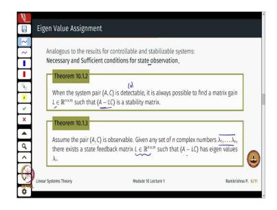
So, very similar to what were the conditions here right what was the necessary conditions for A, A - L C to be here. Stability matrix was that the this pair A and C must be detectable. Or observable in our case right or when the pair A, C is observable then I can place all the eigen values of A - L C at the this desired locations right.
