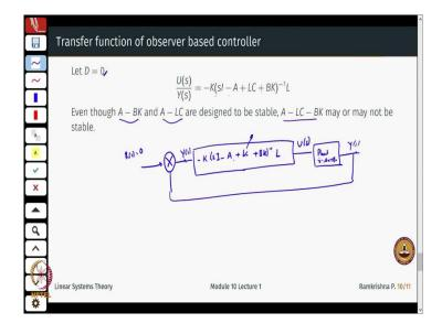
And what you also what we also saw at the end was that the design of the controller and observer. Do not actually interfere with each other and this is how the how the closed loop in terms of a of a transfer function looks like right.
