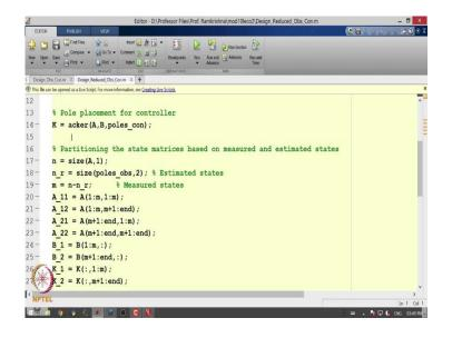
Then I just do the sa[me]- same thing for k to find the controller gain that will be the same ah. And then now I design a reduce observer based on the states which look like this right. So, I have to now design sorry design an observer for. Or in other words I can also say that I want to design a full state observer for a system which looks like this in  $x_2$  right and a certain output here right.
