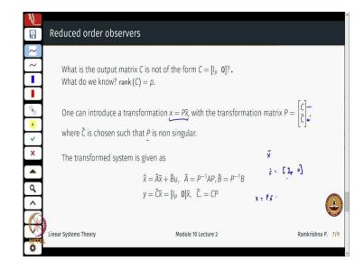
So, what if the output matrix is not of the form  $[I_p \ 0]$  well, we know what is the rank of C right rank of C is p. And therefore, we use a standard trick of coordinate transformation that let  $x = P\bar{x}$  be a transformation with P given by C. And then  $\tilde{C}$  and then  $\tilde{C}$  is chosen such that P is full rank that as in the same way as we did for the observer decomposition or the even in the dual way the controllable decomposition.
