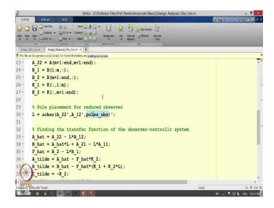
Design an observer for this  $A_{22}$  minus this pair  $A_{22}$ ,  $A_{12}$  and this we know was observable right. And I just run the code for, so the observer design for this pair  $A_{22}$  and  $A_{12}$  with the poles being at -8, -8. And the rest of the process remains the same.
