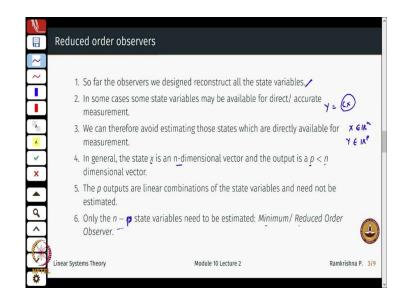
In the observer design so far what we saw was that, we reconstructed all the state variables ok. So, in some cases some state variables might be available for direct or even accurate measurement. And therefore, one can avoid estimating those states right. So, whatever is available for measurement, we can just directly measure those and feedback and whatever are not available for measurement we can possibly construct an observer.
