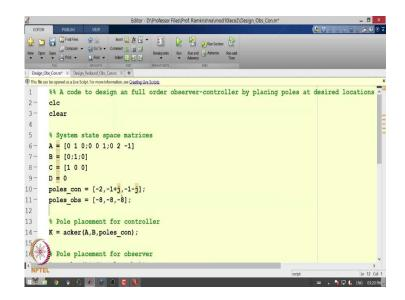
Now, ok, so, MATLAB gives you bunch of tools to do the pole placements. So, I will just use the command for ackerman's formula. So, I have A; which is my system matrix which is defined by this thing over here. So, I have B which is the input matrix I know what are the desired poles? So, once you just give this three inputs. So, this command here it will it will plot it will show you what are the what is the controller gain similarly for the observer gain.
