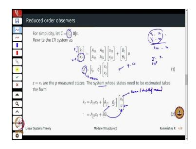
So, let us see how this works ok. So, let us for simplicity say that p variables are of the form or the p outputs or of the form  $y_1 = x_1$  till  $y_p = x_p$  ok. And the remaining once are the once which I which I need to estimate I do not know what is how does  $x_{p+1}$  one look like till  $x_n$  right. But I know how  $x_1$  till  $x_p$  looks like right I just making a very nice assumption here that this holds.
