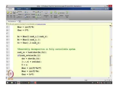
We will take the controllability part. And then we will take an observable decomposition on the fully controllable system. So, this is what we do. (Refer Slide Time: 10:08)
