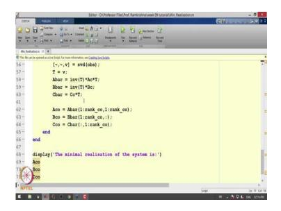
And if the rank is less than the full rank, then again we do again we find out the observability matrix then we take the svd of the observability matrix and then transform is follows. So, this code will run the whole thing, I already copied the whole model into this variable call ss underscore models. So, I will run this code and you will see what happens.
