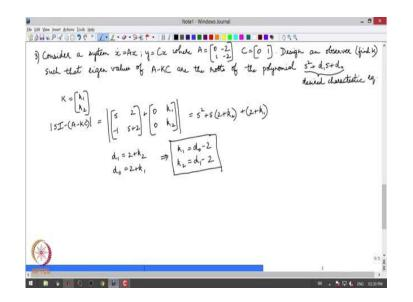
So, in this problem we are asked to design an observer which means we need to find an observer gain matrix K such that we have a system  $\dot{x}=A x$ , and y = C x. And we want to place the eigenvalues of the observer a -K C such that they are the roots of the polynomial  $s^2 + d_1s + d_0$ . So, this is the desired characteristic equation.
