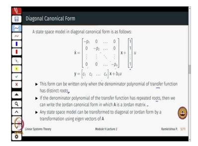
So, an interesting aspect is the diagonal form right, where I can just split the A matrix into the diagonal entries which are the eigenvalues of the A matrix. And, well and interesting to note is that if I write the system in the diagonal form, it is easier to check controllability because as you I have all non-zero eigenvalues on the diagonal, then the system is controllable if and only if each entry of the U matrix has a has a entry one right or a nonzero entry so to speak right.
