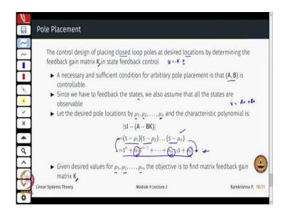
So, this technique is called the pole placement technique right so which essentially means we are placing the poles or the eigenvalues of the closed loop system at some desired locations or some predefined locations ok. So, the control design problem is of placing the closed loop system at desired locations by choosing an appropriate feedback gain matrix K right, and then just applying this control law u = -K x ok.
