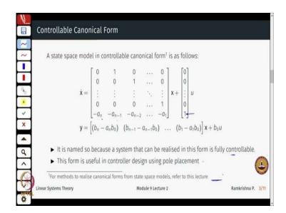
So, I have something like this. So, the controllable canonical form would just be like this at its  $\dot{x_1}$  is  $x_2$ ,  $\dot{x_2} = x_3$  and so on and  $\dot{x_n}$  will have all the coefficients of the denominator terms over here, and the input will just disappear in the last entry of the B matrix ok. It is named this way because if I can write a system in this form it is always fully controllable.
