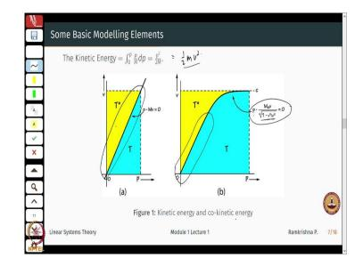
Now, and then I can derive the kinetic energy to be  $\frac{p^2}{2m}$  right and this is  $also\frac{1}{2}mv^2$  of what I learnt, because of the linear relationship between the momentum and the velocityok.
