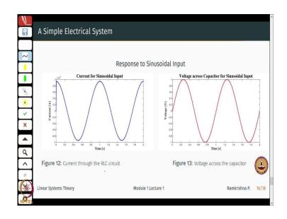
So, I also know that a good or a typical behavior of linear systems is if you; if the input is sinusoidal, the output is also sinusoidal.WhatI do much of thiswe did while we were doing the frequency response; bode plots and nyquist plots and things like that. So, this also we know right that the input to a sinusoidal signal, the output will be a sinusoidal signalwith a little change in magnitude and phase and that will depend on my parameters R L and C of the circuit.
