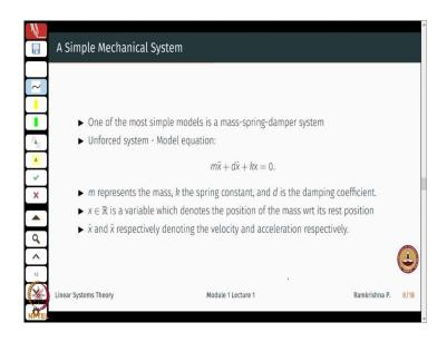
So, one of the simplest example is of any mechanical system which will have a kinetic energy element, which will have a potential energy elements say a spring and some kind of friction in the system and any mechanical system typically can be modeled in this way right. So, m is a certain mass,k is a spring constant, d is damping coefficient and we are not looking at any external forces. I am just looking at a plane autonomous system with x
