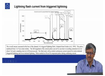
little more than 100 milliseconds and M components, this slow varying pulse superimposed on the continuous current.
