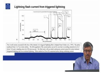
is a current that is measured at the base of the channel, actual lightning current during one of those trigger lightning.
