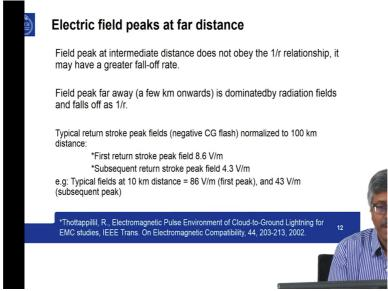
Now electric field peaks at far distance. Field peaks at intermediate distance does not obey the 1 by r relationship and it may have a greater falloff rate where as field peak faraway is dominated by radiation fields and falls off as 1 over r.
