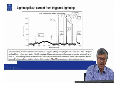
is the initial continuous current process of few hundreds of ampere in amplitude. This is the so-called stage immediately after the wire (()) (09:53) where there is a continuous current. This part is only present in upward initiated lightning or in triggered lightning.
