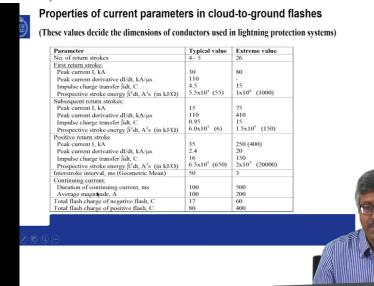
So the properties of current parameters in cloud to ground lightning is summarized here. So you can use this for reference. What is shown here is the typical value or some sort of an average value and what is shown here is extreme value that is maximum value that people have measured with real lightning.
