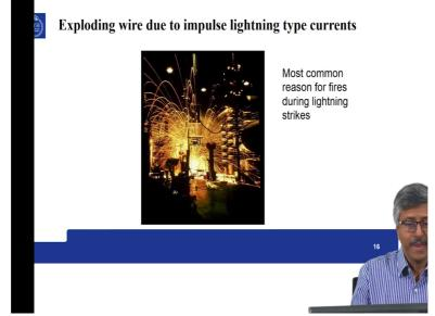
First of all, the exploding wires due to impulse lightning type of currents because of the enormous energy the wires may explode. This is an experiment from a high voltage lab of wire exploding when you subject it to lightning type of currents.
