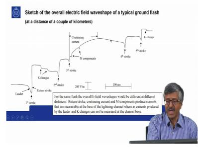
then again a fourth stroke then again a fifth stroke then some rearrangement of charges in the cloud then finally the flash gets extinguished. The whole process is less than 1 second.
