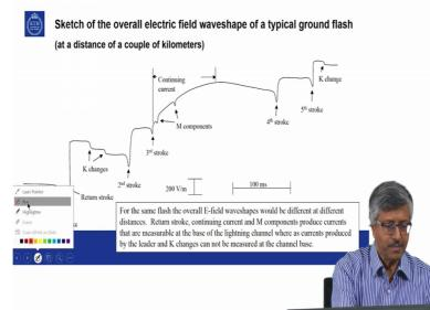
so as lightning is coming down from the sky, first it is in form of a leader. That you will not be able to see with the naked eye. As it is approaching the ground it will create the electric field change that goes in one particular direction.
