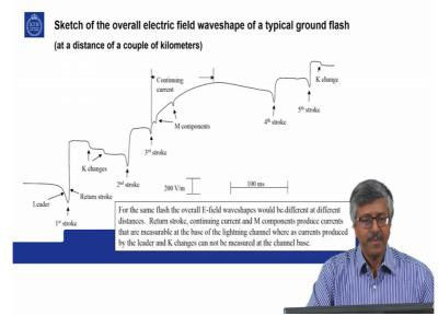
What is shown here is the overall sketch of vertical electric field wave shape of a typical ground flash at a distance of couple of kilometers.
