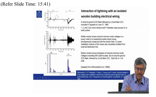
is a cloud flash. It has no connections to the ground. This happens in the cloud only. So what is interesting is that even though all these pulses, bipolar pulses are happening in the cloud, the structure is responding to this and you can find how many pulses exceeded 80 volt peak to peak over here
