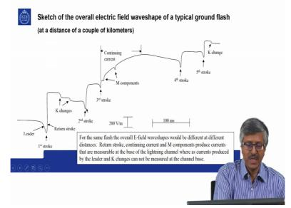
The second stroke in microsecond scale then after that again you have a dark period then along the channel the third stroke, well obviously this stroke
