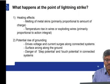
So what happens at the point of lightning strike? So one is the heating effect. Now because of the large currents and temperature.
