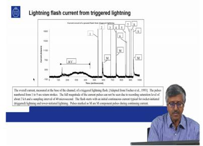
Previously we have seen the process of triggered lightning by shooting a small rocket upward with a trailing wire. And lightning can be artificially triggered with those type of technique from thunder clouds.
