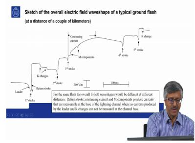
so this is how the electric field change will look like during a return stroke. So the rise time here is just a few microseconds only.
