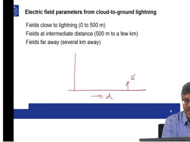
And close to the channel and faraway channel E is proportional to 1 over d,
