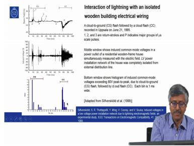
So the conclusion from this is that any lightning that happens, whether it is cloud to ground or cloud to cloud, you know the structure is responding. But usually it is cloud to ground lightning that is more of a threat because this is now more than 20 kilometer away.
