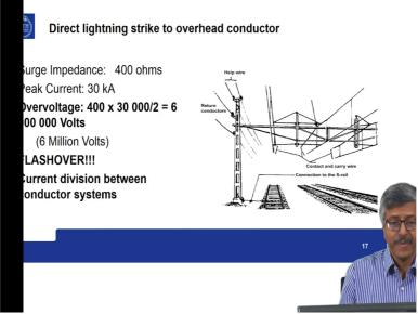
And does lightning strike to overhead conductor? Suppose, so this is a railway line. These lines may have surge impedance of the order of 400 ohms. Assume that your lightning has a peak current of 30 kilo ampere, the average current.
