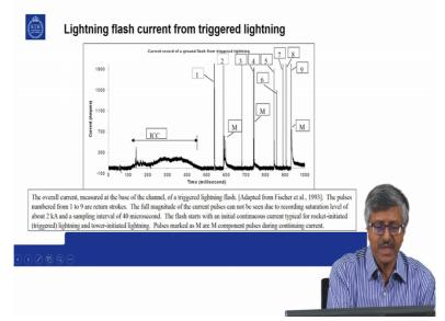
here it is in millisecond up to 1 second is shown, the current is in amperes, up to 2000 amperes are shown. Now these pulses 1, 2, 3, 4 like that most of them are above 2000 amperes but it is kind of cut, to show the finer details of low currents.
