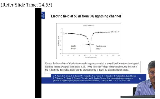
Electric field very close to the lightning channel, a picture is shown here. So you have the leader that is coming down. And now here this is in microsecond scale. Because you are so close to the channel, it is only a distance of 50 meter so this is the last several meters that you are seeing. Then you have the return stroke.
