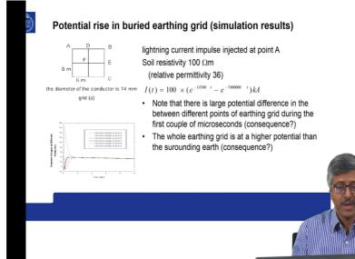
So this phenomena can be illustrated by a simulation. So typically in substations, power substations. We have substation mat in the form of a grid underneath the substation buried so that the 50 Hertz power supply.
