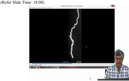
So only some of this brightening are return stroke. Others are just pulses coming down the channel called M components.
