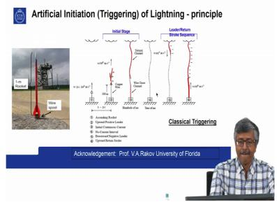
Lot of studies on lightning are done by artificial initiation of lightning by shooting small rocket upwards, and these rockets carry, carry a wire pole at the end.
