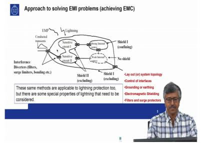
We have seen that the generic approach to solving E M I problems for achieving or achieving E M C, we have seen about zoning principles, that is system topology, control of interfaces, grounding or earthing, electromagnetic shielding, filters and surge protectors.
