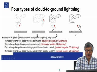
Now these are the four types of cloud to ground lightning. So based on the initial direction of the leader, you call it as downward lightning or upward lightning, 3 and 4 upward lightning, these are downward lightning.
