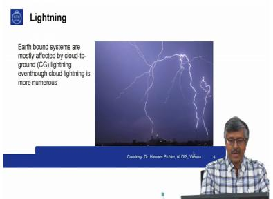
So earth bound systems are mostly affected by cloud to ground lightning. Even though cloud lightning is more numerous.
