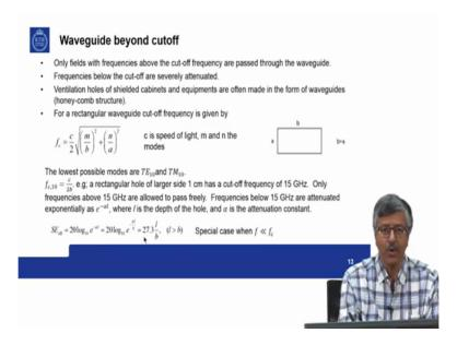
Now waveguide beyond cutoff, the principle is like this. Suppose you have a rectangular cross section waveguide and it has got a depth of length l, the length of the waveguide, now b is greater than a let us assume, only fields with frequencies above a particular cut-off frequency are passed through the waveguides and all those frequencies below that cut-off frequency will be attenuated.
