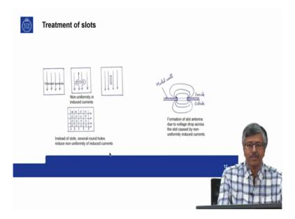
Then if you have slots the orientation of slots become important and if you know that induced currents are in this particular way this is not and if there is a slot like this the induced currents are non-uniformed and that will create the potential difference across the slot and you will create a kind of a slot antenna due to the voltage drop across so this will radiate both to inside and outside and create problems.
