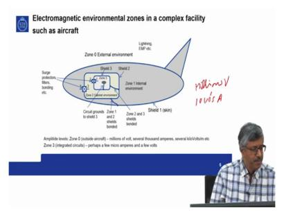
Now the above concept is described more carefully in this picture, so this is picture of an aircraft, here you have zone 0 external environment lightning, EMP, EMP is from (())(9:02) portion electromagnetic pulse that is zone 0 and zone 1 is internal environment, then you have a shield 2 again excluding kind of a shield, then you have shield 3 and here you have very sensitive flight control (())(9:27) things.
