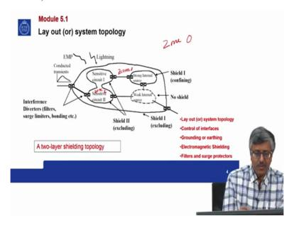
Now we take module 1, layout or system topology. Now assume that you have a area where you want to protect the system inside you want to protect from external electric and magnetic fields, so this is the area boundary. It can be an airplane or it can be a shielded enclosure or it can be a just a room where you have some sensitive equipments. So outside you have several harsh electromagnetic environment both conducted transients and radiated transients can get into this area.
