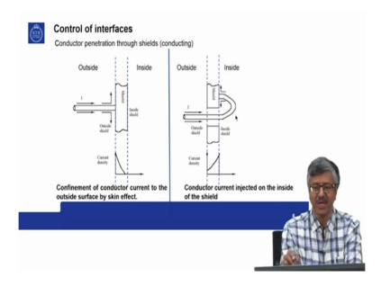
Now how do we control the interfaces? Because you can create different zones, you can bond the boundaries of the zones together if they are metallic, but often you want to have conductors penetrating it. So it can be grounding conductors, it can be insulated conductors, it can be water pipes, heating pipes, gas, communication cables, so how do we control that? So as much as possible you want to keep the zone boundaries separate.
