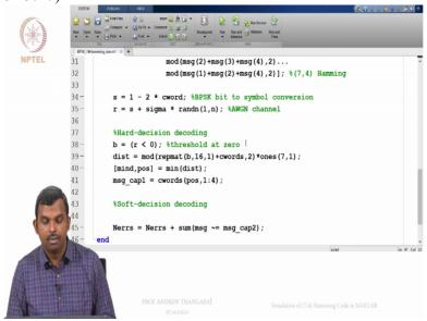
So hopefully it was clear to people. I wrote it down a bit quickly. Think about what I am doing. I am finding the distance between b and every possible codeword and finding that codeword which is closest minimum distance between this and that, Ok. So let us do, so we will run this. I mean I have to check if I have made any mistakes or not. Maybe I made a mistake.
