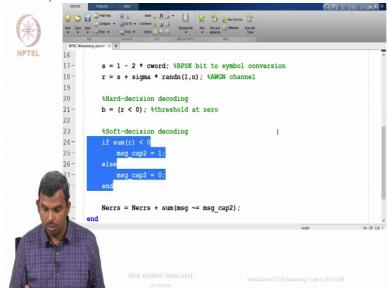
this cannot be the same. This will have to be real out, Ok. Remember what we do in hard decision decoding, you have to find the distance of the hard decision vector b from every codeword and find that codeword which is closest to it, Ok. So that is the task in hard decision decoding.
