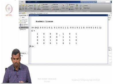
so you can check. This is the generator matrix that I had before, alright. So now I have to multiply with the message bits. How many message bits do I have? I have 4 message bits so there are 16 possible binary vectors. So how do you get a list of 16 possible binary vectors? So it turns out that there is this little command here which I use. There are, I am sure other possibilities here.
