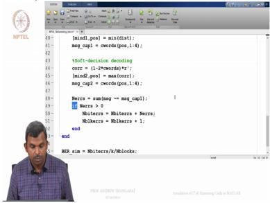
So once again what I am doing here, I am looking at if there was an error in this block. If there was an error in this block I am incrementing N block errors by 1 and then N bit errors by number of errors, Ok.
