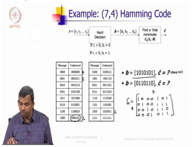
is actually m, m the second message bit XORed with the third message bit XORed with the fourth message bit, right?
