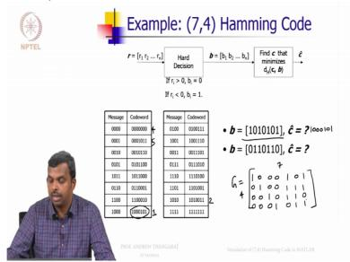
so this is the generator matrix for this 7 4 Hamming code. So you have, when you multiply m with G with the message bits appearing in the first 4 locations and then the first parity will be m 0 plus m 1 plus m 2. The second parity will be m 1 plus m 2 plus 3. And the third parity is m 1 plus m 2 plus m 4, Ok.
