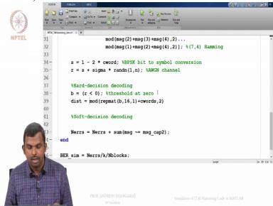
So this is just the XORs, so how do I find the weight? So it turns out you can multiply a vector on the right, Ok and this will give me the distances,
