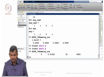
So we get point 0 1, there were 4000 bits that were transmitted. Remember we had 1000 blocks of 4 bits each, codeword is 7000 bits but then, 4000 bits were the message bits. There were 61 bit errors and you got this.
