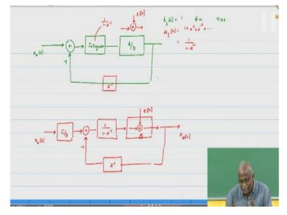
So, here is a modified quantizer, I have the analog signal xa of t, this is going to be the C to D type of quantizer, so I am going to precede the quantizer so basically, we will think of it as instead of C to D as an A to D converter so basically, it is a finite number of bits conversion apart but I am going to precede it with a integrator okay. I am going to precede it with an integrator, so what is an integrator?
