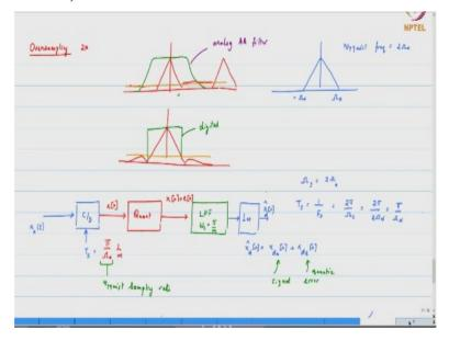
So over sampling, how can over sampling help and what are the ways in which we can leverage it, we can take advantage of it okay, so over sampling basically means that we can when you do the representation, the copies of the spectrum now come further apart right that is what is the; so let us take the a simple case that I do 2x over sampling, now this is where you will start to see the benefits of what we have done what we have discussed okay.
