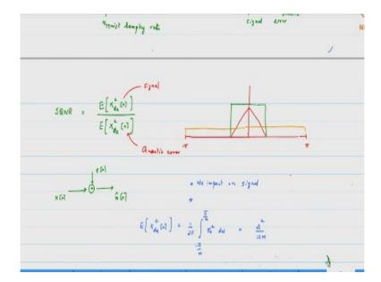
So, the signal to quantization noise ratio now becomes SQNR is expected value of x da of n whole squared that signal power divided by expected value of x de squared of n, so that is the signal component, this is the signal part, this is the quantization error part okay, quantization error okay, so here is where I would need you to visualize the process as follows, so the pictorial representation of this is the following.
