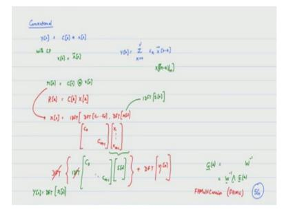
So, this is the conventional thought process, conventional okay, conventional says input-output relationship is always a convolution okay, C of n convolved with x of n, x of n you have put in redundancy whatever it is you want to do, okay now, if I have done cyclic prefix with CP, I hope you will recall that x of n with CP actually becomes looks like a periodic signal, we call it x tilde because you know the data kind of looks like wraparound.
