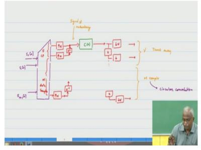
The insertion okay, the insertion of the cyclic prefix, so that happens through the multiplication with the Fcp matrix, so we can see that is happening by adding some new entries at the top then you make it in from parallel to serial that is becomes a signal with redundancy passing through the channel, channel will do linear convolution that is always the case.
