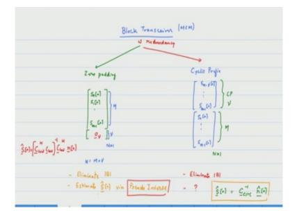
So a good way to visualize the introduction of redundancy in the transceivers that we are working with is; one is zero padding where we add the zeros, the number of zeros must be at least equal to the number of channel taps that you have in your signal, it cannot be less it can be more but at least and because we want the redundancy to be as minimum as small as possible, we want to keep it to the length of the channel time.
