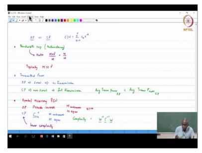
So zero padding versus CP. Are there any advantages disadvantages of each of those? So in both cases, the channel length is the same C of z. C of z is=summation K=0 through nu C subscript K z power -K that is the same. The bandwidth expansion in both cases that is the amount of redundancy that we have introduced, bandwidth expansion that is another name for redundancy, both cases we have used the same amount of redundancy.
