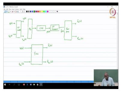
We take a vector of data S0 of n SM-1 of n okay and then we do the cyclic prefix insertion, CP insertion which means basically this will become a larger vector okay. So this becomes the X vector, X0 of n Xn-1 of n okay, that becomes my then I combine it to pass it through a channel. So this is where the unblocking occurs, the parallel to serial conversion okay. So take this information basically we have inserted the cyclic prefix.
