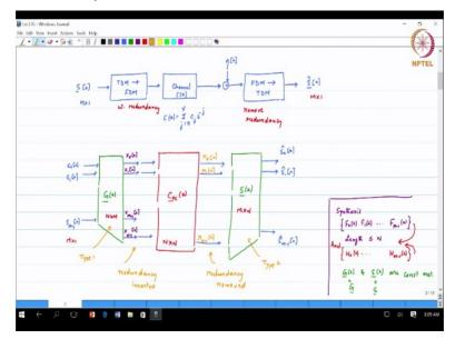
So we have dispersive channel which has nu + 1 taps, so effectively it is a ISI channel with nu symbols of ISI. We want to introduce redundancy, so at the transmitter we want to introduce redundancy. Therefore, upsampling becomes by a factor of N. So the channel now becomes encapsulated in the form of a pseudo-circulant matrix which dimensions N x N. Then, at the receiver we want to remove the redundancy and then extract out the signals and this is the broad framework okay.
