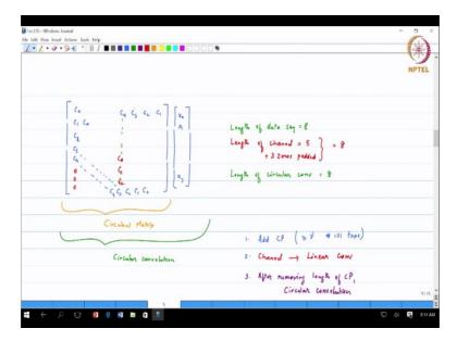
So this is how the circular convolution comes about. So the cyclic prefix is very important for us to be able to generate the circular form and once you get it into this structure, we also recognize that this matrix is circulant and by definition will also be Toeplitz in its form okay and we will take advantage of that okay.
