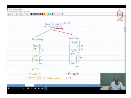
Now what we said was in the context of the block transceivers, so in the framework of the diagram in the previous slide, we call that as a block transceiver okay. It is also intended to be a multicarrier modulation. Basically, our intention is to extract them and it is also with redundancy okay. So this is the broad framework that we are doing. One approach that we have seen is the zero padding approach.
