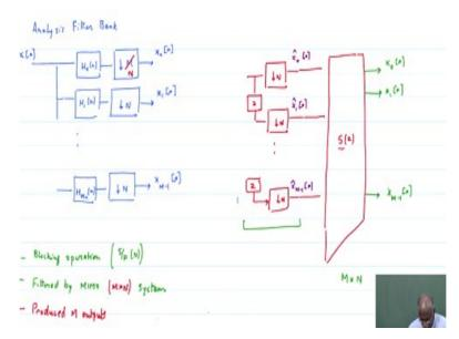
Now analysis filter bank we said we will do a Type 2 polyphase decomposition. So basically this is the structure of the polyphase decomposition of the analysis filter. Since you have up sampled by N which means introduction of redundancy you must down sample by N in order
