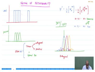
Now redundancy along with that comes the notion of orthogonality basically we want to be able to establish these signals independent of each other these narrow band signals. So we are looking for ways of separating them. Of course separating them in frequency is one way and there are other way by which you can say that okay as long as they do not overlap there is a notion of orthogonality in frequency I should be able to separate.
