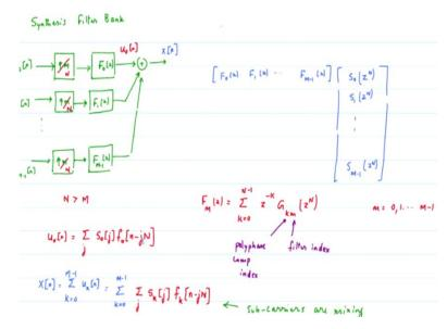
So with this configuration we said how will the synthesis filter bank look because that is the first stage of the transmultiplexer. Up sampling by M followed by the filter that is a minimal configuration, but we introduce up sampling by N by the same filters, but now these filters have to be slightly differently designed, but that part it will come later. So the vector representation is a scalar F0, F1 up to F M-1 multiplied by these signals which are up sampled.
