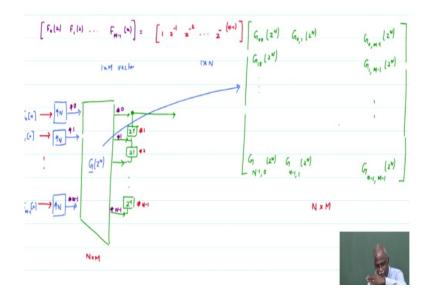
Once you did the polyphase decomposition we showed that the synthesis Filter bank can then be represented in this form where G of Z is a rectangular matrix. You are splitting each filter into N polyphase components there are M of them. So basically the polyphase component of each filter are along the columns and there are M such filters and therefore you get a N\*M basically the redundancy part is being shown by a trapezoid instead of a rectangle.
