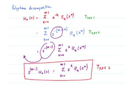
So just a quick definition Type 1 you have powers of Z power –k that is a delay chain sequence of delays. The Type 2 has a series of advance operator. So again Type 1, Type 2 was reviewed.
