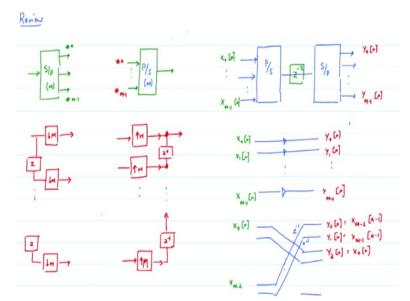
We also received the blocking and unblocking operations. The blocking operation the creation of blocks happens through a advance chain by down sampling we call this as the blocking, the reverse operation as the unblocking operation with the delay chain. And we said that using the results of up sampling followed by a delay followed by down sampling there are certain simplification that we can achieve if you did not have the Z power -2 these would be straight lines.
