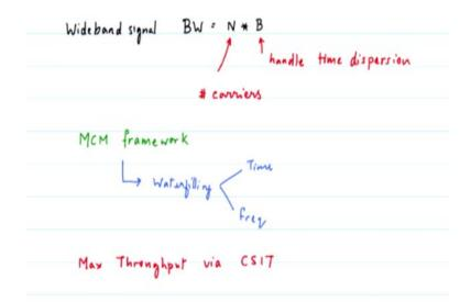
And the motivation for Multicarrier modulation is stems from the fact that we want to deal with wideband signals so that is primarily our interest. A wideband signal has several challenges you get frequency selective fading and the complexity of equalizer is quite a challenge. So we said that the wideband signal we will treat as N narrow band carriers N\*B. So this is where the Multicarrier modulation concept is coming from.
