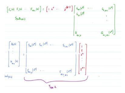
Last review portion of this thing is that we wrote the polyphase implementation the matrix representation of the synthesis filters. These are the synthesis filters followed by the analysis filters very important.
