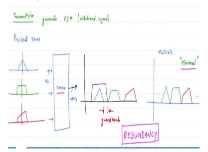
Now on this side if each of these is Ns and you have M of them and because of the up sampling this becomes M times Ns so that is a minimal transmultiplexer. So minimal transmultiplexer is one where you have, but if you did up sampling by N so with redundancy we are increasing the number of resources. So it is N times Ns where N> M so somewhere the notion of additional resources comes in the minute.
