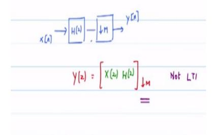
If I fed in X of n to H of z followed by a down sampler and this is Y of n I say oh good I already know how to analyze this, this should be Y of z= X of z, H of z down sampled by M, but I am not able to pull X of z out. So this is not LTI because when I down sample X of z I will get all the shifted version. So this is not LTI because I cannot take out X of z. So again notation actually comes in a very handy and useful manner, but actually when you start using it actually becomes more beneficial.
