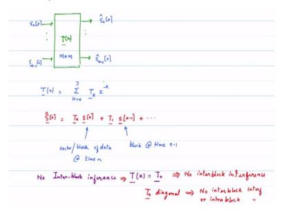
I am going to go back to this particular representation which means that I have a matrix T of z M by M matrix where each of the entries are T00 of z, T01 of z all of those are matrices. I have M inputs I have M outputs this is another interpretation again very importation that you are comfortable with this as well S0 of n all the way to S M-1 of n S0 hat of n, S M-1 hat of n input output relationship indicated by this M \*M matrix.
