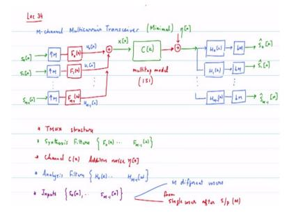
Okay so back to the reference figure I will have to keep switching back and forth. This is my reference figure okay. Reference figure from here this is the synthesis filter, pass through the channel I mean ignoring the noise for the moment, passing through the analysis filter. Now given the result that we have just now studied can you tell you what is the transfer function between S0 of n and S0 hat of n.
