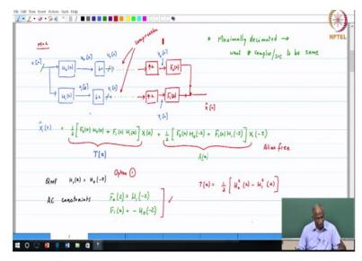
Maximally decimated basically means that whatever is your input sample rate, number of samples per second will be the net sample rate across these different subchannels. If you did not do the downsampling by a factor of 2, you can find that if you split it into 2 channels, the number of samples per second will go, so maximally decimated, one of the key reasons is because we want the sample rate to be the same.
