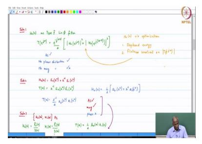
This is more of an overview, so the first solution, solution 1 where we have implemented the aliasing cancellation and the QMF condition, you have got T of z of this form. The first solution was; let us design H0 of z as an FIR type 2 linear phase, type 2 linear phase filter okay. Then, what we get is the transfer function T e of j omega is=e power -j omega N/2 mod H0 e of j omega magnitude squared+magnitude H0 e of j omega –pi whole squared okay.
