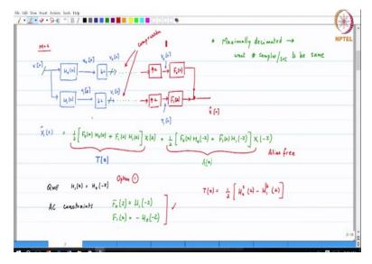
Which one is it? It will be a half band filter, which you will design with the appropriate attenuation and scaling. Then, take its spectral factorization that will become H0 and then the mirror image filter, not exactly the QMF version, but you will want to make it the para conjugate becomes H1. Then, correspondingly F0 and F1 are chosen to cancel aliasing. Then, you are guaranteed that the input-output is in the form of a delay LTI system which gives you perfect reconstruction.
