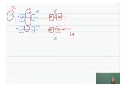
So, the 2 channel case this input signal X of n which we split in through a low pass and a high pass signal. We call that as X0 and X1 and down sample each of them called V0 V1 then you know there is processing but we said that in the analysis stage we are saying that we are not considering the processing, it is basically those signals are connected to the synthesis filters up sampling by a factor of 2 filter filtering through F0 and F1.
