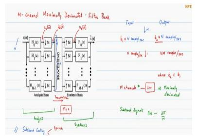
This is the M channel general setup as we mentioned yesterday is different from a trans multiplexer, the conventional approach is that in a filter bank typically the analysis filters come first followed by synthesis filter. In a trans multiplexer they are reversed in terms of position because you have the synthesis happening first but again from a view point you can study it as a trans multiplexer or as a conventional filter bank.
