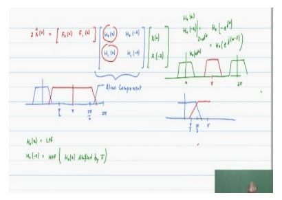
So, supposing I do a I do a 2 channel split okay, so I will write down all the filters there is a filter here and there is a down sampling by a factor of 2, okay now I split only this branch as one more stage down sampling by a factor of 2, and this is down sample by a factor of 2, so now if you look at it. looks like you have different down sampling in the different branches because you have a 4. in the upper two branches and two in the lower branch.
