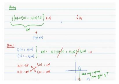
So the aliasing term, if you go back and look at the last equation that we wrote the aliasing term consists of H0 –Z F0 of Z + H1 of –Z, F1 of Z you can have a half or not does not matter may be just put a half also there, this whole thing if we call that as A of Z there is some transfer function times X of - Z. This is the contribution of X of – Z to the output so basically this is what will show up at the output of X hat of Z.
