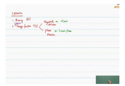
So, to summarize the key points are that we have three types of distortions in a two channel filter bank, the first one is aliasing distortion that is represented by A of Z only if A of Z is 0 then we can talk about the other one then the transfer function becomes T of Z if A of Z=0 then the transfer function now is T of Z, which can have magnitude distortion you want to eliminate this you need to have an all pass function.
