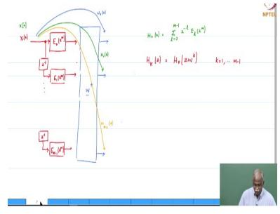
The general framework of a DFT filterbank, so keep this as a useful reference point so this would be a DFT filterbank and key elements are the fact that we have done the polyphase decomposition and have shown that the inverse DFT is the one that appears here. So we call it the DFT filterbank. We come back to this particular concept several times but right now in this particular discussion specific discussion we are interested in the concept in the context of the spectral analysis.
