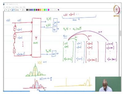
So we went so far as to say that the basic structure of the DFT that we compute, you take a stream which is in the form of x of n, x of n+1 you take a block M and then you compute its DFT and that block can be generated by means of passing the input signal through a series of
