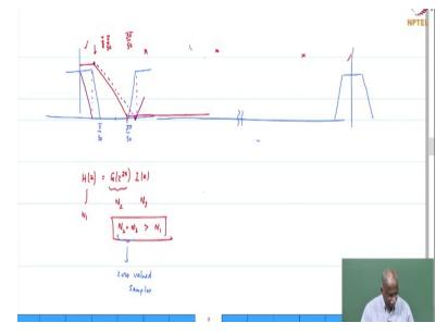
So after the up sampling by a factor of 50 there is a cut-off there is first image at pi/50. Where is the next image? 3pi/2 is the next frequency edge that divided by 50 so 3pi/50 is going to be the next edge. So let me just show it as this here. So this is going to be 3pi/50 that is the up sampling by a factor of 25 is going to produce images and it is going to produce several images, okay. And we just want to sort of leave the all of these and then go all the way to the last image.
