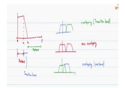
In the last lecture we introduced the notion of filter banks and we said that we would like to get several filters which span the range from 0 to 2 pi and in that context we showed that there are types of filter banks if the adjacent filters have some overlap that is the most traditional or most commonly encountered. Occasionally you may want them to be non overlapping or you may want to have significant amount of overlap.
