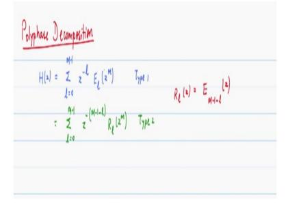
We have two types of polyphase decomposition usually the Type 1 polyphase decomposition associated with the down sampling or with the analysis filters. Remember we talked about when a signal gets split that is called the analysis filter. So usually Type 1 is associated with analysis filters Type 2 is associated with the synthesis filters. Again we will see several cases of these and then it will become familiar with that.
