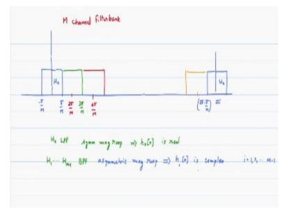
So therefore the uniform filter bank that we are talking about has the following structure. If it is a M channel Filter bank that means the range from 0 to 2 pi will be divided into M filter of equal bandwidth and they are obtained by the shifts using the complex exponentials M channel Filter bank. And this turns out to be very, very interesting and very rich area and we will spend quite a bit of time studying and analyzing this particular case.
