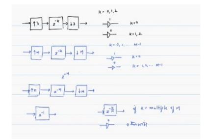
Supposing I have the following set up and I have up sampling by a factor of 3 a delay Z power -K and down sampling by a factor of 3 and where K can be 0, 1 or 2. The output is if K=0 you know up sampling, down sampling cancel each other. So this will be equal to the identity system with gain 1 for K=0 so that is equal to gain of 0 for K=1 and you can also verify that for K=2 is also going to be the same case.
