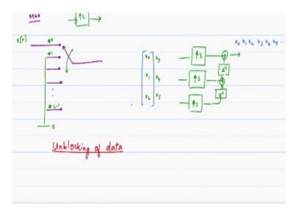
Now the counterpart the up sampler we said that can be viewed as a multiplexing operation where L-1 0 valued samples are being fed in which is indicated in this one and of course if you combine the up sampler with the delay elements this would give us the parallel to serial conversion, this would be the parallel to serial conversion in this case with L = 3 channels with the anti-clockwise commutator okay.
