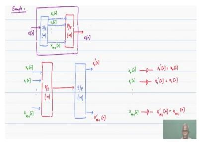
So example of what we have just looked at currently. So example 1 applying the concepts of multiplexer and demultiplexer. I have X of N. I am going to introduce a serial to parallel conversion of order M okay, which means that I will have M streams coming out, I would just like, for convenience I would represent them as X0 of N, these are the subsequences X1 of N and the last one as XM - 1 of N, M parallel sub sequences okay.
