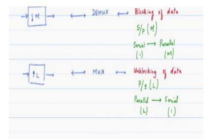
That we said that the down converter or the down sampler down sampling by a factor of M we said was related to a demultiplexer, one that split a high rate stream into multiple low rate streams out of which one of them is being kept. So it has the view of demultiplexer and we also saw that this has the same role as blocking of data, creating blocks of data, blocking of data.
