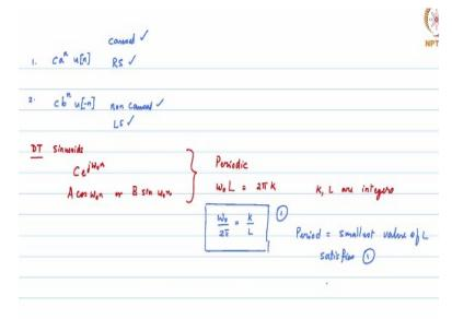
If I have a complex exponential, c a power n u of n okay, so this would be causal yes and right sided of course, causal means it would be right sided, the other one would be a second example would be c times b power n u of -n, this is left sided clearly and it is not anti-causal, it is non-causal, okay because it has got, it is defined at n equal to 0 again, the same property that we discussed earlier.
