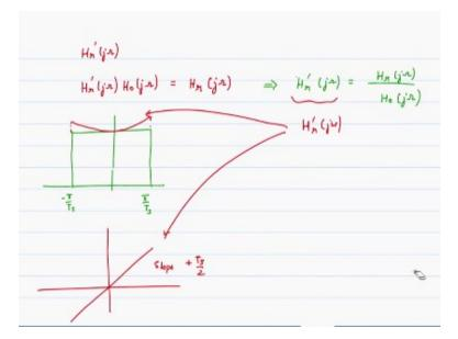
But we need now need to use Hr prime of j Omega and the condition on Hr prime of j Omega is that Hr prime of j Omega since it is a cascading of filters multiplied by H naught of j Omega must be equal to the ideal reconstruction or I would like it to be as close to the ideal reconstruction filter as possible okay, so this basically tells me that what is the response of this Hr prime because now we have to design Hr prime to be equal to Hr of j Omega divided by H naught of j Omega.
