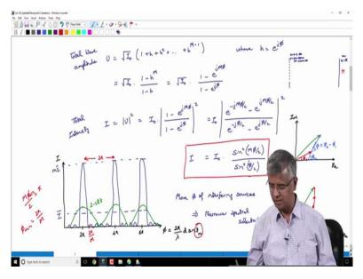
So I can make, in the same structure I can make a Fabry-Perot Etalon just by doing this. So let us go ahead and try to see how this structure can give this bandpass filter characteristic. So, to analyze this structure what do we have to rely on? We go back to this sort of an analysis we did previously - where we have multiple beam interference.
