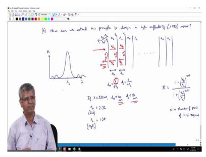
Can we use this principle now to make a high reflectivity mirror? So that is the second part. Question is - how can we extend this principle to design high reflectivity? High reflectivitylet us say greater than 99 percent mirror. So, if that is what we want to do, how do we go about doing that?
