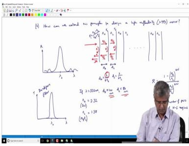
Can I do some trick over here with this structure, with this principle such that - instead of getting a reflection like this, I get a transmission over a narrow wavelength range around a particular  $\lambda_0$ ? Okay, is it possible to have something like this? So what type of filter would you call this? Band pass filter right. So can I extend this concept and find a way to get a band pass filter?
