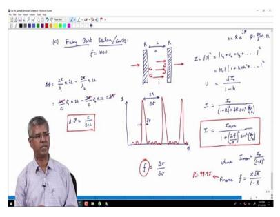
So overall what we are set to do is a Fabry-Perot Etalon or Fabry-Perot Cavity using this thin film interference concept. So what we have said is - we have assumed that we are going to be able to make one mirror here and another mirror here and light that is getting into the cavity is coming here. It is going through reflection, it is coming back reflection and it is coming here and then that is undergoing one more reflection and coming back and so on right.
