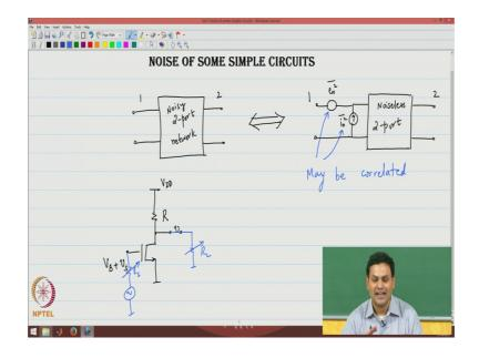
Let us say this is a noisy 2 port network and the input port is port 1 and the output port is port 2. Now it turns out that this is exactly identical to a noiseless 2 port with its noise referred as a noise voltage and a noise current at the input and I will call those input referred noise sources as e n squared and i n squared.
