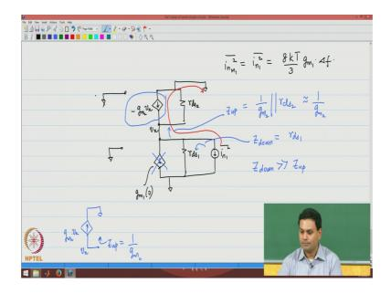
So, to understand this a little bit further we will need to draw the small signal equivalent circuit I will call this intermediate node voltage as V x and therefore, this current source for M 2 is minus g m 2 times V x because the gate is a small signal ground.
