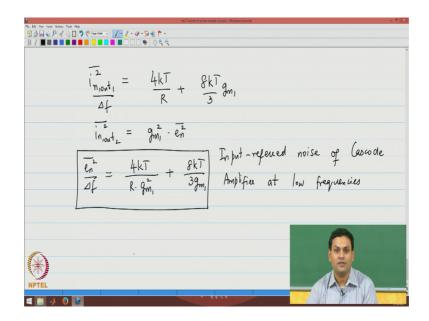
And therefore, now we can write the total noise current at the output which is 4 k T by R plus 8 k T by 3 g m 1.
