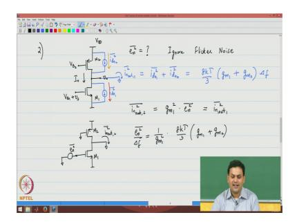
The noise current flowing through the output is increasing. So, it may seem at least at the beginning on the phase of it; it seems a little bit counterintuitive. But please note that the noise current squared increases linearly with g m, but the output signal increases as the square of g m.
