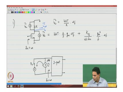
We can now say that the input referred noise can be calculated by considering all the noise sources in the circuit when you are doing noise analysis the input source does not matter. So, we will ground. So, the input not a signal of interest we are only interested in the noise signals inside the circuit.
