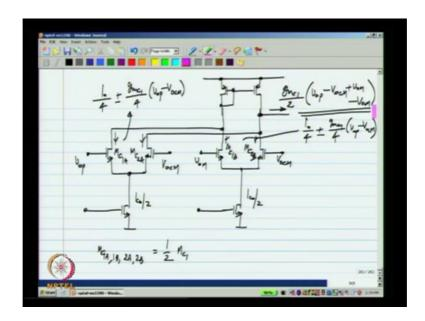
. So, what I will do is, I will have two differential pairs VOP and VOCM, VOM and VOCM and I add up the currents. Let us I have IC 0 by 2 flowing here, IC 0 by 2 flowing there and then these transistors; let us say each of these transistors is half the size of the M Mc 1 used in the previous circuit ok. So, we have half the current of before and half the device has us before when I say half of Mc 1 half the width ok. So, the gm of these transistors is gmc 1 by 2 ok.
