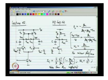
. So, first a quick review of very simple, this is the fully differential single stage opamp, when this part is the trans conductor and when loaded by capacitors, it becomes an opamp. These are the two register are the common mode feedback detector. Now the differential equivalent circuit is very simple ok.
