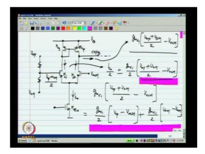
This is because it is just more complicated to draw, but you will get the point even without the buffer. The part that I am going to draw now is a common mode detector itself plus the single stage single ended opamp used for feedback. So, this is the common mode feedback that goes to M3 and M 4 ok.
