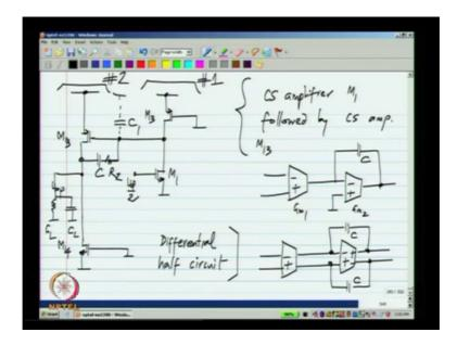
So, we will have M1 with its source grounded M3 with its gate grounded, and this is M 13 and M 14 ok. So, this is the output. So, this is the posting input Vd by 2 and this is the output VOP. This is the differential half circuit of the fully differential two stage opamp, this is the first stage and here we have the second stage ok.
