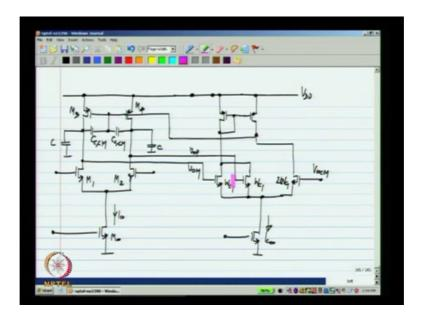
This is one of the differential pairs and this is the other differential pair add up the two currents together and whether in to the other side, I also add up these two currents ok, and this is the output of the single ended opamp, which is used for common mode feedback. So, we complete the feedback loop in this way. The rest of the circuit remains this same. The CC CM is the integrating capacitors if you want to think of it that way.
