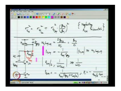
It will be equal to sigma VT 1 square with this is the mismatch between the transistors M 1 and M 2 plus the mismatch between the transistors that formed the load times gm 3 by gm 1 square ok. Again I have negated the contributions from R the mismatch in RCM, well contributed to the overall offset, but because the value of RCM so large that can be neglected.
