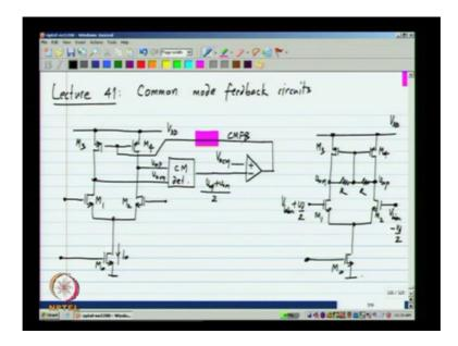
This is our single stage opamp and the voltage here at the gate of M3 and M4 controls the values of the current sources from the top and at the tail, I have assumed the fixed current source I naught.
