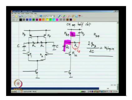
Now, if we go back to the very simple common mode feedback, we had earlier all way had was this R connected there, there will be invariable. Be some parasitic capacitance at this node due to this transistors as well as may be due to the resistors, ok? A common mode equivalent circuit of this is, ok? So, there may be some parasitic capacitance. Here, I will call at CP 3 and then, to make this into an opamp, we will have the integrating capacitors C, ok? We will have that.
