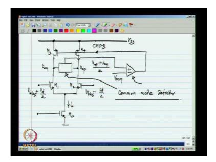
I need detect the output common mode voltage let me call this the common mode detector. So, it is output voltage will be nothing, but V op plus V om divided by 2 then I have to compare it with the desired output common mode voltage V ocm and feed it back to the gates of M 3 and M 4 in the right direction, in the right direction means that if the output common mode is too high what should happen is that what; that means, is that the current in M 3 and M 4 are low lower than the current from M 0.
