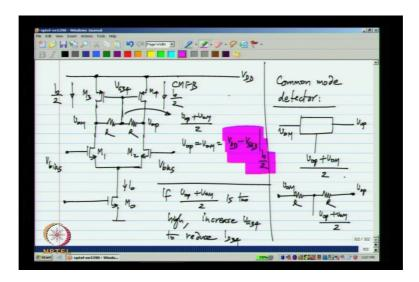
We want to take in V om and Vop and obtain an output V op plus V om divided by 2, how can we do this, the simplest way of getting the average of 2 voltages is to use a resistive divider V op and Vom. So, will get V op plus Vom by 2 if this 2 registers are equal [noise]. So, that is potential candidates for the common mode detector. So, let us use that here we will see what the implication of this is later.
