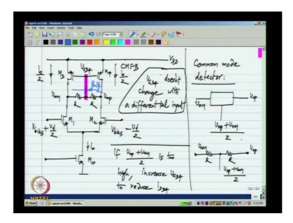
V G3 4 does not change if you have a fully differential input. So, what it mean the that M 3 and M 4 will continued is apply the same current as before and the differential current the extra current that is drawn from M 1 and the extra negative current that is drawn from M 2 will flow through R [noise]. So, there will be a current G m Vd by 2 in that direction ok.
