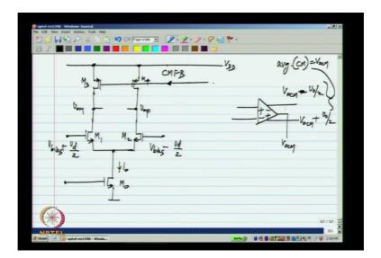
So, let me call this V op and V om we cannot using this kind of biasing this has to come from feedback which is usually call the common mode feedback or CMFB. Now what should this feedback be based on we should based on the average value of V op and V om, we do not want to react to V op and V om individually like that said we need an opamp and opamp output must be able to vary which not that the opamp output voltage must be fixed then the opamp is completely useless.
