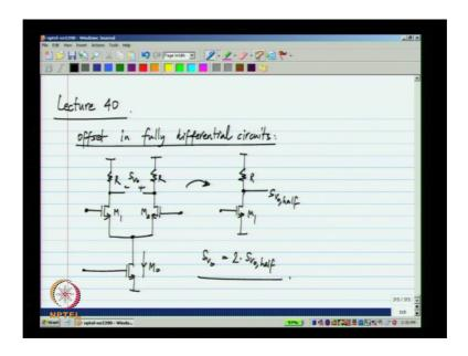
Now we will quickly look at how to calculate offset in a fully differential circuits then move on to design fully differential opamps [noise]. Now we saw that if we have a fully differential circuit such as the differential pair loaded by the resisters the differential noise voltage between these 2 notes will have some spectral density S vo. Now we take the half circuit and calculate it is output noise voltage spectral density let me call it S vo half S vo will be 2 times S vo half.
