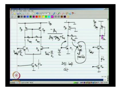
This is my fully differential of opamp or the simplest realization of the fully differential opamp and the differential half circuit is given by only one half of it by grounding all the nodes along the line of symmetry this is the differential half circuit and the common mode half circuit is obtained by folding the 2 halves together which gives me M 3 4 and R by 2 and M 1 2 and M 0 and here we just have V bias [noise].
