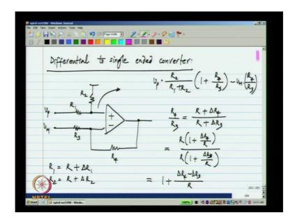
Now, this is the circuit that is used very often to convert the difference voltage into a single added voltage. So, if we have two large voltages V p and V m and you want to take the difference between them you can use this circuit and you can see that the output will be exactly equal to V p minus V m. So, what is the catch here?
