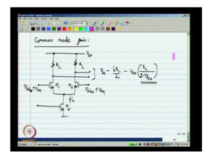
We have already looked at a common mode gain of a stage like this loaded by R L we know that if we apply a small single common mode voltages to the two sides; the outputs will rise up together and the common mode gain will be this is approximately the common mode gain I have ignored the g m s of M 1 and M 2 are assume that the output resistance of M naught is so, large that the common mode gain can be approximated by R L by 2 time rds 0.
