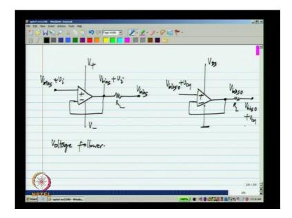
Now let me take a very simple amplifier which is a voltage follower now what does it mean to say that I can have a single supply or dual supplies first of all what it means is I can have any value of V bias here and V bias is there and I can apply an input signal and output here will be at the same V bias plus V i.
