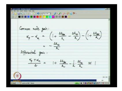
So, the common mode gain of this circuit is alpha p minus alpha m which is equal to 1 plus delta R 3 4 by R minus delta R 1 2 by R minus alpha m which is 1 plus delta R 3 4 divided by R and it turns out to be simply minus delta R 1 2 divided by R and the differential gain which is alpha p plus alpha m divided by 2 this is the number that multiplies V p minus V m and that is equal to 1 plus delta R 3 4 by R minus 1 by 2 delta R 1 2 divided by R.
