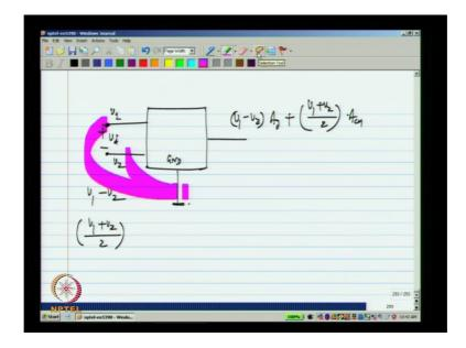
Now all circuits will have some common reference point which is the local ground of the circuit and what you really respond to is individual voltage is V 1 and V 2 with respect to ground. Now you design circuit. So, that it respond predominantly to V 1 minus V 2 and it does not respond to V 1 plus V 2 by 2 as we have discussed earlier we can think of the voltages V 1 and V 2 individually or as the difference and common mode voltages.
