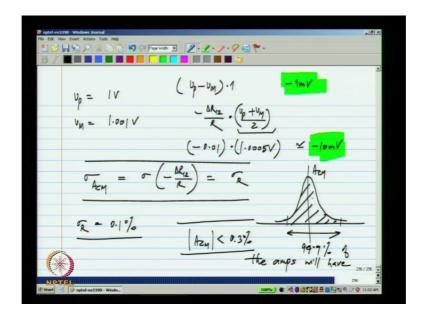
So, let us a inputs are 1 volt and 1.001 volts. So, the output will be V p minus V m times 1 this part is minus 1 mill volt plus some resistor mismatch times V p plus V m by 2. Now V p plus V m by 2 is approximately 1 volts it is 1.0005 volts so in fact, let me write that here. Now how much is delta R 1 2 by R it depends on the physical size of the resistors that you use.
