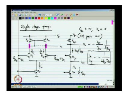
We do not have resistors, but we have a current mirror load, let us say again we apply only a common mode small signal input that is identical inputs to the two sides of the differential pair. Now how do we figure out the what the output voltages first of all we know that when the circuit is perfectly symmetrical that is M 1 and M 2 are identical M 3 and M 4 are a identical the voltages here and there will be exactly identical.
