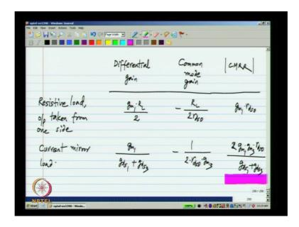
Now let us say we have a differential pair with a resistive load and output taken from one side the differential gain will be gm 1 R L divided by 2 and the common mode gain will be R L by 2 rds 0. It will be negative and if you have a current mirror load the differential gain will be gm 1 by gds 1 plus gds 3 and the common mode gain will be minus 1 over 2 rds 0 gm 3 and the contrast is obvious.
