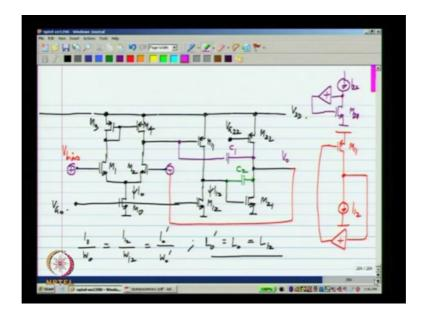
Similarly if you think of a M 22 and M 21; M 22 is a current source I 22 and this is M 21. So, that again the gain from here to there is negative and gain from there to there is negative it is a common source amplifier. So, we have a positive incremental gain amplifier connecting that way. And we know that if we do that M 21 is a negative feedback and a current of I 22 flows through that.
