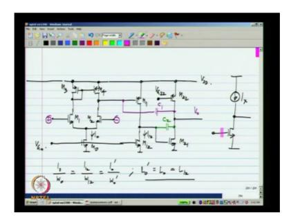
So, first of all as I have been mentioning several times the gates of a M 0 and M 22 and M 12 and so on are not connected to fixed voltages, they are always derived from current mirrors. Let me call this M 0 prime and this is I 0 prime ok; as usual whenever you make a current mirror, you make the lens of all transistors the same and the widths are in the ratio of the currents that you found.
