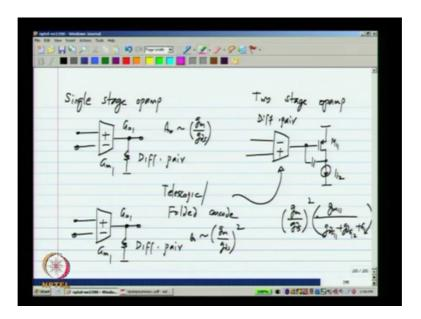
We have a single stage Op-Amp of some G m 1 and this is just the differential pair; it has some G o 1 and the DC gain is of the order of G m by gds of a single transistor.
