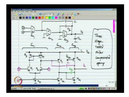
We know that at the signal level; what we need are three stages; this is the input of the Op-Amp and that is the output. We can think of it as the input G m 1 driving a current controlled voltage source with a transadmittance SC or a transimpedance 1 over SC and the current controlled voltage source is made using this two stage Op-Amp.
