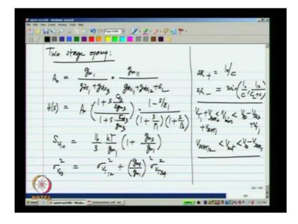
So, to summarize the two stage Op-Amp has a DC gain which is the product of the first stage and the second stage gain. And the important thing is that even if you have a
