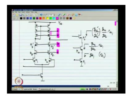
I will show it for the telescopic cascode topology; now to just to illustrate the principle; I will show also a just common source amplifier. Looking in here that is why this is M 1 I will have gds 1 as the output conductance or rds 1 as the output resistance; if I cascoded with MC the output resistance will be gmc by gdsc times rds 1. I could cascoded with one more transistor that is why M C prime the output resistance will be gmc prime by gdsc prime; gmc by gdsc times rds 1.
