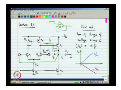
V naught is changing at a rate of I naught by C; now what does it mean? The voltage across C L which is V naught is also changing at this rate. So, the current through C L is the slope of this voltage times the capacitance. So, the current through C L would be C L times I naught by C. Similarly if the output voltage was reducing; if the output voltage was doing something like that with the slope of minus I naught by C, there would be a current in the other direction.
