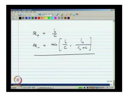
So, in the two stage Op-Amp the positive slew rate is I naught by C and the negative slew rate is whichever is smaller of I naught by C and I 12 by C L plus C. So, there are
