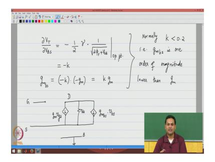
What about dou V T over dou V BS? Dou V T over dou V BS is clearly minus half gamma times this expression this is of course, calculated at the operating point, so V SB value is chosen to be the DC operating point value to calculate this expression therefore, I am going to x call this sum factor k because gm bs is finally, minus k times minus gm which is k times gm.
