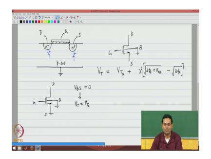
How is the device made if I were to draw the cross section of the device? If I look at the MOSFET I need the 2 drain source diffusions I will take the example of an NMOS transistor. So, they will be n plus diffusions on the p substrate, I will denote that by p-sub and I will grow the gate oxide and on top of that the polysilicon will be the gate, so I will denote these by this three the gate drain and the source.
