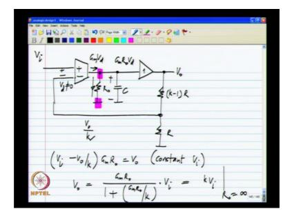
Vi minus V naught by k and that times Gm Ro is the voltage developed across the resistor and that is the same voltage that is given out as V out. So, this is equal to V naught ok.
