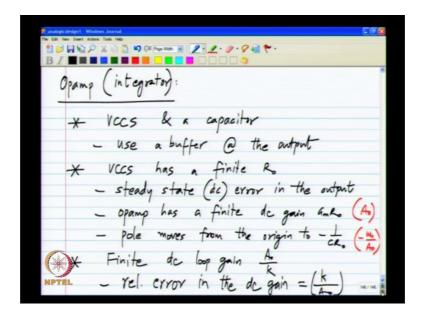
So, to summarize, to implement an op amp which is an integrator, we need to have some integrating function and which we do using a Voltage Control Current Source and the capacitor and we also use a buffer at the output. So, as not to disturb the currents flowing through the capacitor due to the load.
