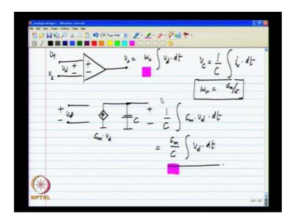
Now, a capacitor integrates the current flowing through it ok. Whereas, we want to integrate let me call this V 1 and V 2 and the difference is Vd. These are the inputs of the op amp as we have defined it and we want to integrate Vd to get V owe would like Vo to be some omega u integral of Vd with respect to time ok.
