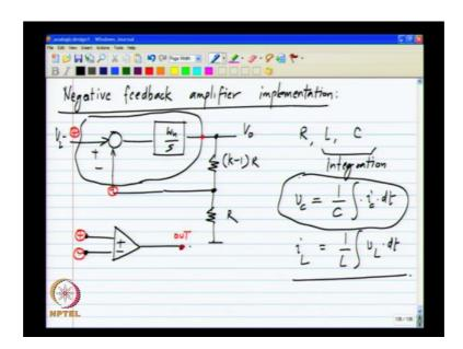
So, as you know this is an amplifier of gain k and we have investigated its behaviour extensively able to implement. This we need to have way to take the difference between the input and the feedback quantities and a way to integrate it ok. And this combination of taking the difference and integrating it, we know is the op amp or the operational amplifier. So, this corresponds to these terminals; we can think of this as a plus terminal minus and this is the output.
