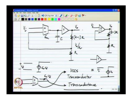
And, we know that our amplifier has to look like this 1 there are many kinds of amplifiers you can build, but will still take our prototype amplifier that we started with; the amplifier of gain k ok. Here, we have to have our resistive divider and this is Vd and I will use the simpler notation of simply writing Gm, but it is understood that the current here will be Gm times Vd ok.
