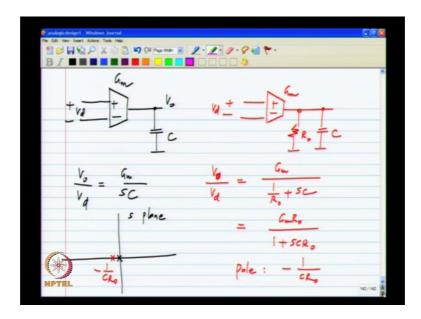
So, if you look at the s plane originally the pole was here and now, this can be written as for instance Gm Ro 1 plus S C Ro and the pole is at minus 1 by C R naught ok. So, the pole moves into the left half plane and exactly how much it moves depends on the value of R naught; the higher the value of R naught the lesser the movement into the left half plane ok.
