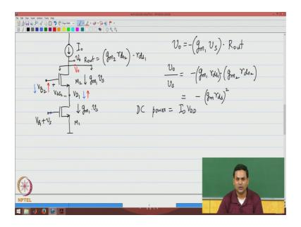
So, let us see what a cascode amplifier will look like if I were to build a cascode amplifier, I have a single current source I naught I will again call these devices m 1 and m 2 and I am going to apply a bias voltage V B 1 an appropriate bias voltage V B 1 plus the signal at the gate of m 1.
