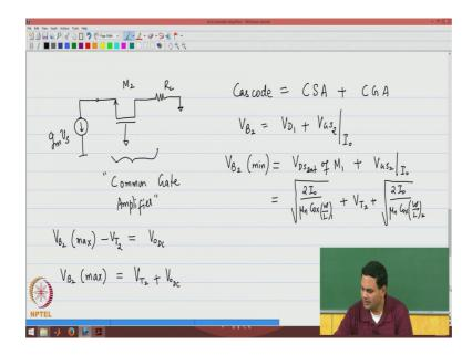
If I were to redraw it slightly differently this is device m 2 the input for device m 2 is basically the signal current of value g m times V g g m times V s and that is the this current source represents device m 1 that creates g m; g m times the s current.
