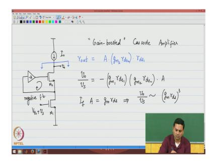
There is one more option to do this I will show that with an illustration on the NMOS cascade. Now in the original cascode amplifier the gate of m 2 was connected to signal ground it was connected to a appropriate dc voltage.
