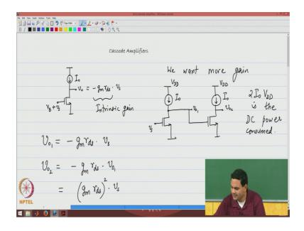
That we have seen before. So, let us assume that the common source amplifier is biased with a drain current of I naught; it has an appropriate gate bias voltage, I will call that V B and along with this I will also apply a small signal voltage V S.
