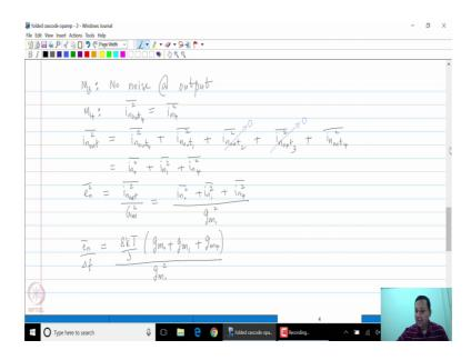
What about M 3? Transistor M 3 is again a common gate structure you do not expect any noise at the output you can follow the exact same procedure and show that the output noise generated by M 3 is equal.
