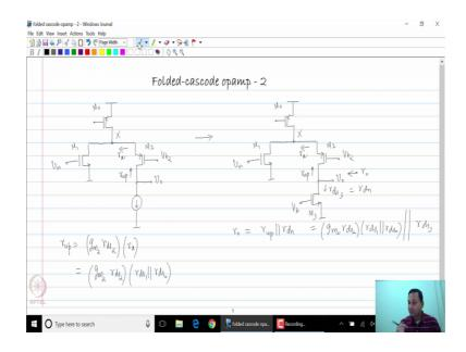
Before we build the full opamp using the folded cascode structure let us take a look at the gain and noise performance of the simple single ended folder cascode structure. So, we will assume that the input is an NMOS anti cascode is a PMOS a device.
