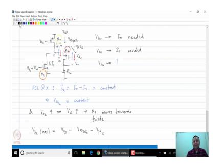
So, let us take this folded-cascode and now let us now modify this because I know that there are no ideal current sources. So, this current source is a bias current from V b flowing into this node. So, that is clearly generated using a PMOS transistor maybe I will call that M 0 and this current is I 0. And of course, the gate of this current source is going to be tied to some voltage V b 0.
