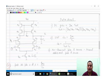
So, now we will take a high swing current mirror the telescopic Opamp with the high swing current mirror and build the datasheet for that particular Opamp. Now let us assume that the currents and sizes are known. So, now, we are in a position to build the datasheet. So, the first characteristics that we are interested in is the DC gain even though I say in DC gain, I want to reemphasize that this is actually the low frequency gain I am not the gain if you apply a DC voltage at the input.
