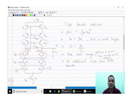
Next I will also find point out that it is possible to build what is called a triple cascode amplifier. So, similar to the telescopic amplifier with a single cascade device, it is all it is also possible to add double cascode or a triple cascode device. So, you can add 1 more set of cascode devices on top of the original amplifier cascode to create this amplifier. So, this would have again as you might imagine the game would be of the order of gm rds the whole cube.
