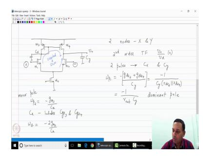
In the case of the 2 stage opamp, let us quickly draw out the picture to draw to understand the analogies. So, if you look at the analogies between the 2 stage opamp and the one stage opamp. So, the one stage opamp have 2 nodes x and y and therefore, it had a second order transfer function. So, its gain had 2 poles. So, 2 poles corresponding to C 2 nodes x and y, they depended on cx and cy they also depend at on the impedance at those nodes.
