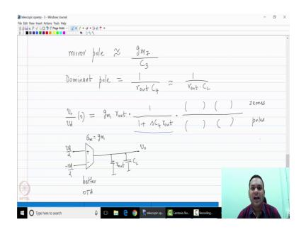
Please note that the mirror pole will be approximately at a frequency that is the impedance at that node or rather the conductance at that node which happens to be one over g m seven we have calculated that in a different lecture. So, the mirror pole will be approximately gm seven over C 3 and this would be one of the important non dominant poles of the system.
