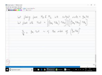
So, the total output currents r is nothing but the total output currents let us call that i out is minus i out from M 8 and M 2 into the output node this is equal to gm 1 times V d.
