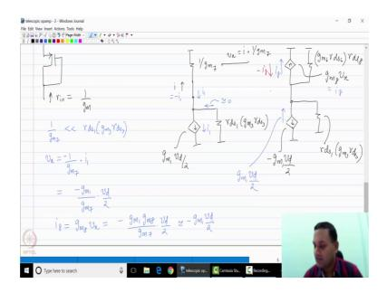
So, this is very similar to taking a common or taking transistor, and connecting it is own gate to it is source it is drain they r in for that 1 over gm. Now it turns out that even for a cascode currents mirror this feedback action gives you input impedance of 1 over gm 7.
