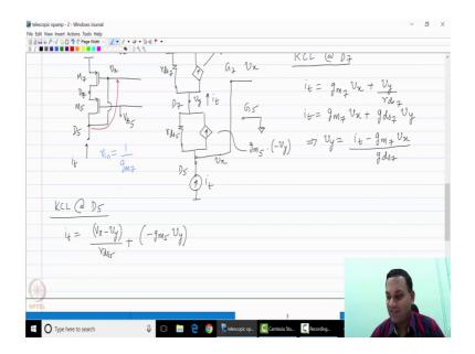
So, please note that the impedance looking upwards r out or r in is 1 over gm 7. Please note that this means that this indicates that there is inherent feedback by connecting the drain of M 5 to the gate of M 7.
