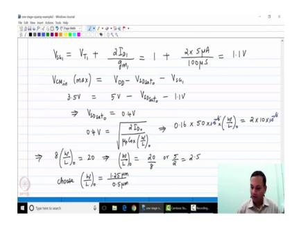
So, V SG 1 is V T 1 plus 2 I D 1 over g m 1 V T 1 is 1 volt plus the current through M 1 is 5 microamperes and g m 1 is 100 microsiemens. And therefore, this is nothing but 10 microamp over 100 microsiemens this is 1.1 volt in such a case the value of V CM in max which is 3.5 volts. So, let us write that down here again is V DD minus V SD sat 0 minus V SG 1. So, 3.5 volts is 5 volts minus V SD sat 0 minus 1.1 volt tells us that V SD sat zero has to be equal to 0.4 volts.
