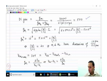
Now, you can see that the DC gain is now larger than expected DC gain is g m 1 by g d s 2 by g d s 2 plus g d s 4. As we have seen earlier, the value of g m 1 was determined to be 100 microsiemens. So, therefore, the DC gain is 100 microsiemen over 0.1 microsiemen plus 0.5 microsiemen, which is 500 volts per volts. We wanted a minimum gain of 100, but we now have a larger DC gain than required which is always better. So, this the DC gain spec is met.
