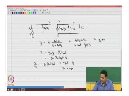
So, the capacitor happens to be a short circuit because it is an infinite capacitor VDD is signal ground. And therefore, the two resistors appear in parallel R A and R B appear in parallel at the gate of the device at the drain is where you take the small signal output voltage and you have two parameters one is R D S the other is g m times V G S, which is the voltage control current source and apart from this you also have the load resistance R L.
