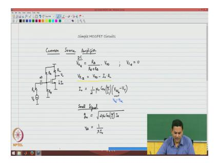
So, let us start of the first circuit that will look at is the common source amplifier. So, I will draw one version as with circuits in general. There are many different versions of the common source amplifier, I will draw the simplest possible version where the source terminal is common to the input and output puts and the drain terminal is where the output is taken and the gate terminal is the input port, where the input signal is applied.
