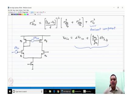
Now, let us try to write down the standard deviation at the input. So, sigma squared o s in is V GS minus V T whole squared V GS minus V T by 2 the whole squared times sigma squared delta R D by R D plus sigma squared delta W over L over W over L plus sigma squared V T. So, this is the expression for the input referred offset of the differential amplifier. And as you can see you expect this to be the dominant component, since it appears directly at the input.
