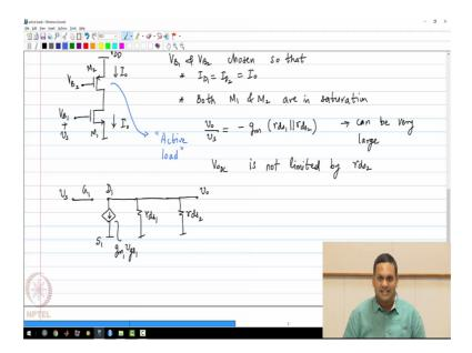
So, this is the amplifier that you have been looking for. So, let us say the NMOS transistor is M 1 and the pmos transistor is M 2 and I am going to say that the NMOS transistor has a bias voltage VB 1 and signal voltage V s applied to the gate, the pmos transistor has some voltage VB 2 at its gate.
