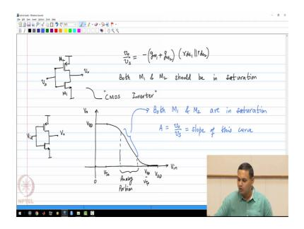
Of course you can also imagine a scenario where you use the pmos transistor for getting some signal gain also. So, what do I mean by that? In the earlier case I was applying V s here and I was connecting the gate of the pmos transistor to small signal ground, but a question can be asked why not connect the gate of the pmos transistor to V s so that you get small signal gain from the pmos transistor also and yes definitely this can be done.
