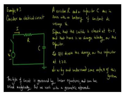
Now let us look at our final example and consider an electrical circuit, so let us go ahead and actually make a diagram of our electrical circuit. We have resistor R and capacitor C which are in series with a battery of constant dc voltage V not. Now suppose that switch is closed at t is equal to zero and that there is no charge initially on the capacitor. Let Q of t denote the charge on the capacitor at the t greater than or equal to zero.
