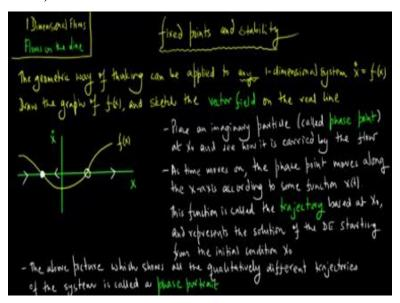
Now welcome back to one dimensional flows, where we are still dealing with flows on the line. The focus of this lecture will be on fixed points and stability. Now the geometric way of thinking can readably be applied to any one dimensional system x dot is equal to f of x. Now essentially you just need to draw the graph of f of x and sketch the vector field on the real line.
