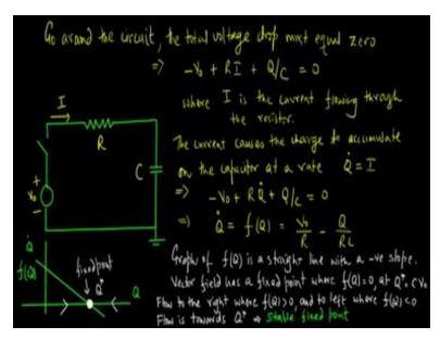
So now, if you go around the circuit, the total voltage drop must equal zero. Which gives us -V not +RI + Q/C = 0. Where, I is the current flowing through the resistor. The current causes the charge to accumulate on the capacitor at a rate Q dot is equal to I, this gives us -V not + RQ dot + Q/C = 0. Rewriting this we get Q dot is equal to f is the function Q = Vnot / R - Q / RC. Now the graph of the f of Q is just a straight line with negative slope.
