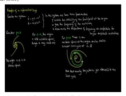
Now let us look at the example of a supercritical half. So, consider the system r dot = mue r - r cube, tita dot = omega + br squared. In this particular system we have three parameters, meu controls the stability of the fixed point at the origin. Omega gives the frequency of the oscillations and b determines the dependence of frequency on amplitude for larger amplitude oscillations.
