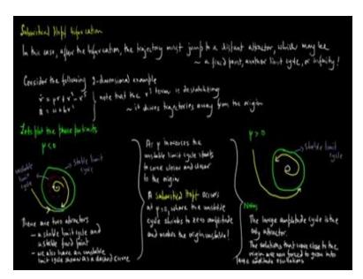
We now consider a subcritical half bifurcation. In this case after the bifurcation the trajectory must jump to a distance attracter which may be a fixed point, another limit cycle or of to infinity. So consider the following two dimensional examples, r dot = meu r + r cube - r5 and tita dot = omega +br squared. Note that the r cube term is destabilising ie it drives trajectories away from the origin.
