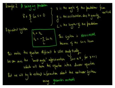
Now let us consider the example of a swinging pendulum the differential equation is x double dot plus g on L sine x is equal to zero. Where x is the angle of the pendulum from vertical, g is the acceleration due to gravity and L is the length of the pendulum. The equivalent system is x1 dot is equal to x2 and x2 dot is equal to minus g on L sine of x1. Now we get to this equivalent system using exactly the same trick as the previous example.
