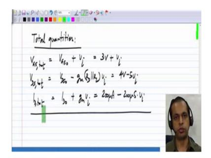
Now to get the total quantities what we have to do is to add the operating point to the incremental quantities  $V_{GS(total)}$  is  $V_{GS0} + v_i$ . In this particular circuit which is 3 volts +  $v_i$  and  $V_{DS(total)} = V_{DS0} - g_m * (R_D || RL) * v_i$  which is 4 v - 5 v<sub>i</sub> and the total drain current( $I_{D(total)}$ ) =  $I_{D0}$
