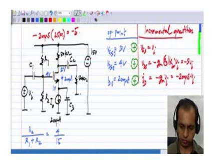
Let me refer to the operating point quantities as  $V_{GS0}$  and  $V_{DS0}$  and  $I_{D0}$ , and the incremental quantities will be  $v_{GS} = v_i$ , because at the gate you have  $v_i$ , the source you have zero, and  $v_{DS} = -g_m^*(R_D \parallel R_L) v_i$ . And this particular case it is  $-200\mu S^*(25k\Omega)^* v_i = -5v_i$  and the incremental drain current  $i_{D=-}g_{m^*}v_i = -200\mu S^* v_i$ .
