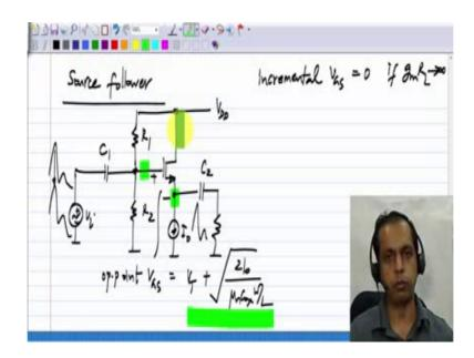
But the same principle applies now what does it means for the complete circuit, let me put down again the complete circuit of the source follower including biasing. This is connected to supply voltage  $V_{dd}$ . First of all the bias point get established and there is negative feedback for biasing itself that is if the actual drain current more than this current the source voltage will increase, the  $V_{GS}$  will reduce. And eventually this operating point gate source voltage will
