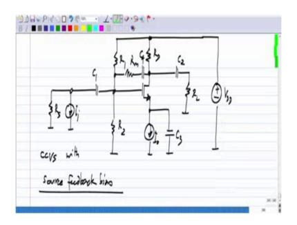
So, this is a current controlled voltage source with source feedback biasing. So that completes the picture of the current controlled voltage source. And we have also illustrated that we can combine at with the two biasing techniques drain feedback and source feedback.
