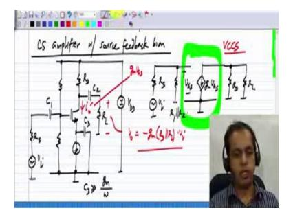
Now this circuit you see is very similar to, let me copy this over, I have copied over the same circuit, and what I want to highlight here is the similarity to a common source amplifier with source feedback biasing. Now, let me go back to that circuit common source amplifier with source feedback bias. What did we have in that case, the only difference between this and that circuit was this  $R_1$  was not their it was short circuited and  $C_3$  was connected directly to
