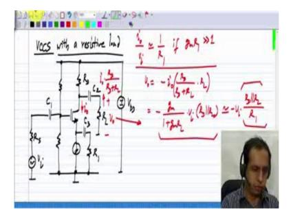
Now, our voltage controlled current source using a single MOS transistor is made like this, we bias it with a current source in the source. And most commonly used way of biasing the drain is through a bias resistor  $R_D$ , and we ac coupled the load to it, and we couple the resistor which defines the trans conductance  $R_1$ , and we also ac coupled the input. Now, the quantity that is controlled by feedback is the small signal incremental current in the drain and
