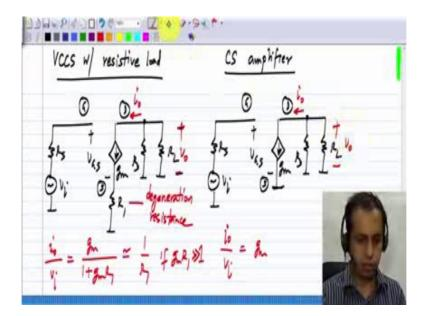
A voltage controlled current source with resistive load, this is used with the voltage output as I mentioned, it looks like, this is  $g_m$  and this quantity is  $v_{gs}$ , these are the drain, gate and source terminals of the MOS transistor. And the common source amplifier is very similar of course, except that the resistance is not there and the source is connected to ground. So, if I
