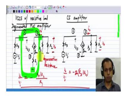
we will have  $\frac{v_o}{v_i} = \frac{R_D \vee i R_L}{R_1}$  in this case, again under this same condition this  $g_m R_1 >> 1$
